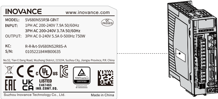
Figure 3-1 Diagram of nameplate descriptions (standard model)
